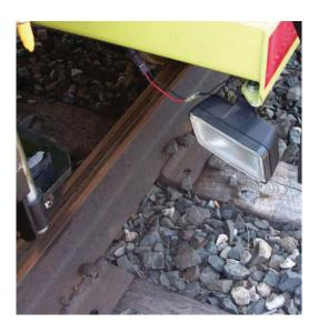
4x6 LED work lights over each rail clearly illuminate the work area, allowing increased precison during anchor adjustments.
