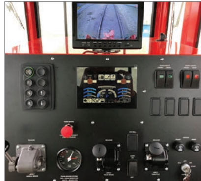
180-degree rotating console with a multifunction display. Dual four-way air suspension seats for operation from either side of cab when in rail mode.
