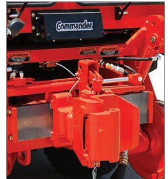
Wide range AAR sliding couplers are air released and hydraulically positioned to improve pulling performance on curves and grades.
