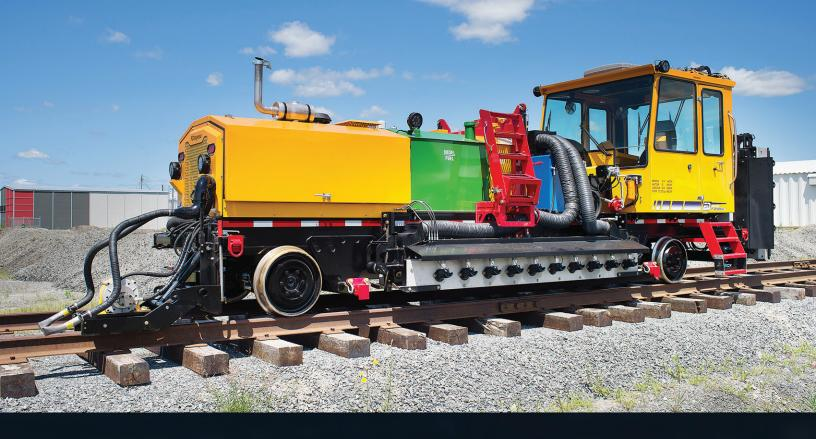
NECESSARY FOR HEATING AND RELIEVING STRESS FROM RAILS
