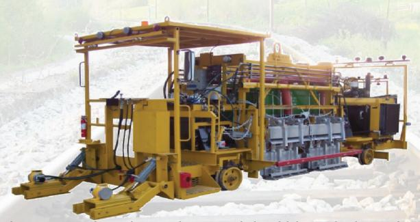
For those situations where safety considerations or fuel availability render the use of propane undesirable for heating continuous welded rail (CWR), Teleweld can provide an alternative.
